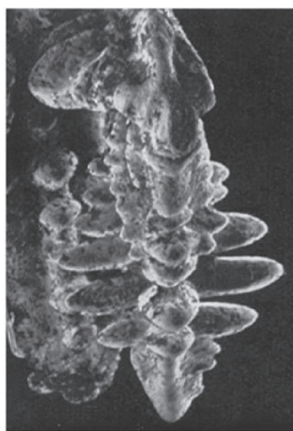
Fig.1: (a) If the liquid is under-cooled, a protuberance on the solid-liquid interface may grow rapidly as a dendrite. (b) Scanning electron micrograph of dendrites in steel.
